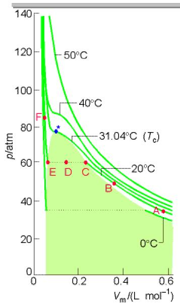
CO<sub>2</sub> gas compressed by a piston at 20°C:
