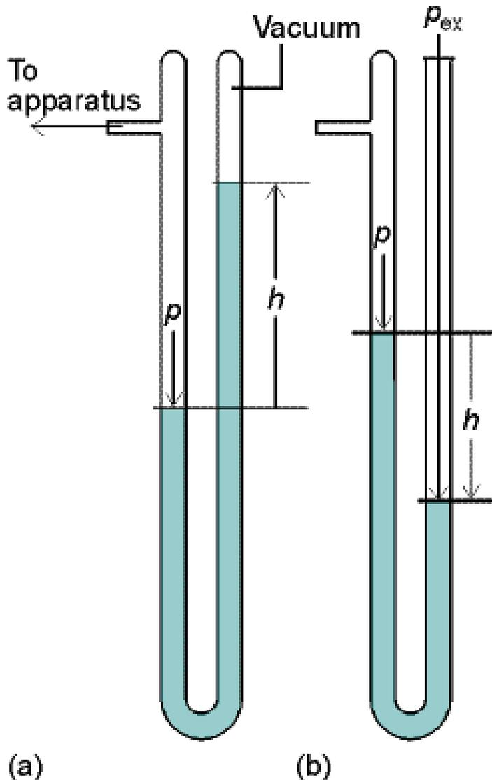
One device used to measure pressure is a **barometer** (by Torricelli). When the column of mercury is in equilibrium with the atmosphere, the pressure at the base is equal to that from the atmosphere - so the height of the mercury is a measure of the external pressure.
